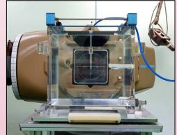
SSDL facility to provide calibrations for dosimetry equipment in KIRAMS Dosimetry Lab
